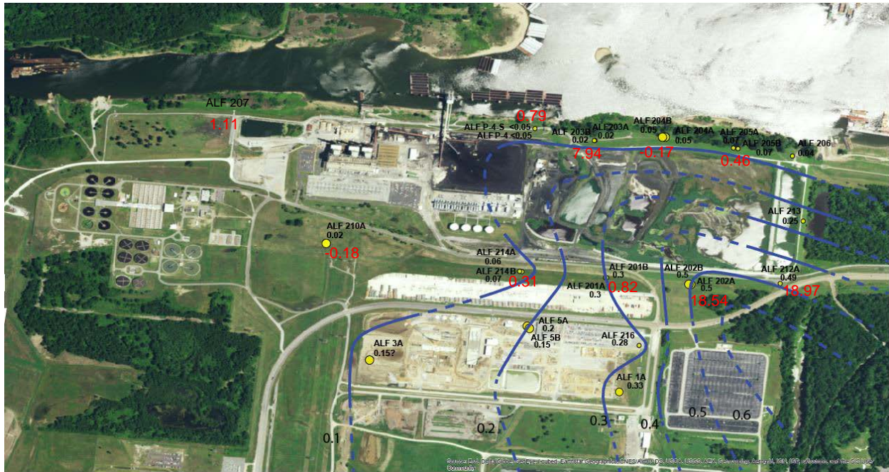
Figure 14 Estimated Drawdown in MRVA Aquifer Monitoring Wells During Memphis Aquifer Pumping Test (values in black, contours in blue). Red Numbers are 9-20-2017 (before Pumping Test) Hydraulic Head Differences between Shallow and Deep MRVA Monitoring Wells (pos. values indicate downward groundwater flow; neg. values indicate upward flow) (from USGS, 2018)
