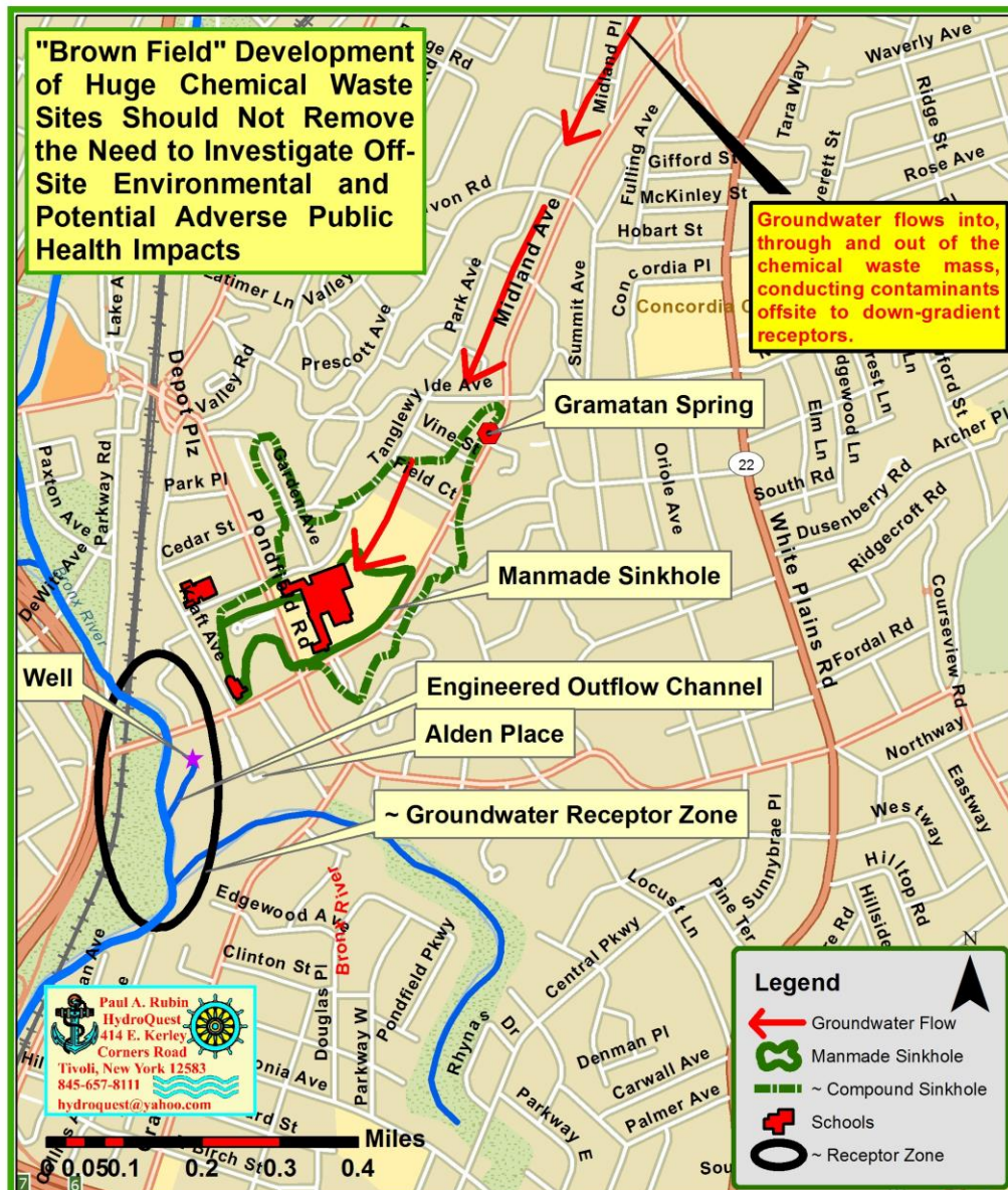
Figure. Hydrogeologically, it is not prudent to leave a huge chemical waste mass within an active groundwater flow system with no knowledge of where contaminants are going or who may be adversely impacted. The former marble quarry on Marbledale Road was filled with massive quantities of chemical wastes, inclusive of volatile and semi-volatile organics, metals, PCBs and more. Waste material is in direct contact with bedrock in an unlined setting with no chemical leachate collection or treatment. Groundwater flow is documented from north-northeast to south-southwest along the alignment of the soluble Inwood Marble. Developing and covering the waste material will not alter or stop down valley contaminant flow. Unfortunately and inappropriately, regulating agencies have not required characterization of off-site contaminant flow routes, presence, type, or concentration. More importantly, down-gradient receptors, inclusive of schools, have not been identified or investigated for potential adverse environmental and health impacts. October 13, 2015
