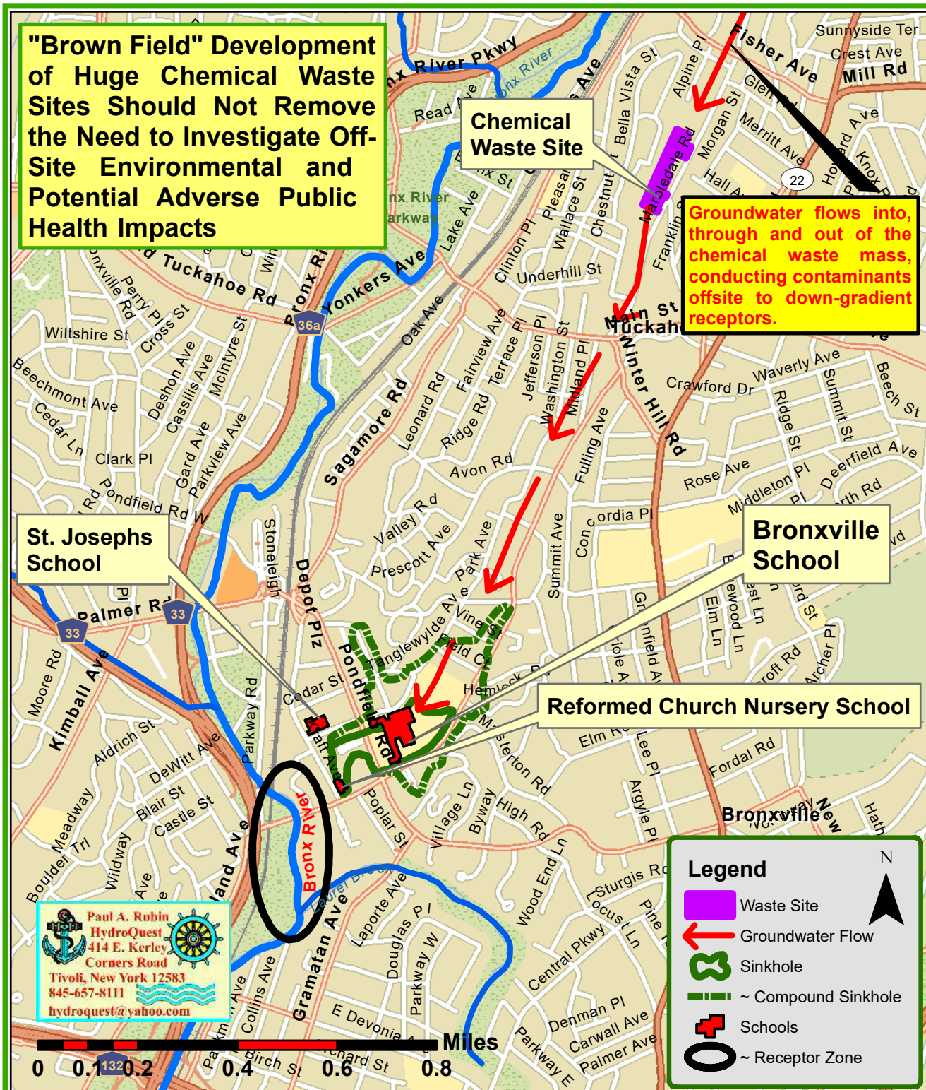
Figure 5. Hydrogeologically, it is not prudent to leave a huge chemical waste mass within an active groundwater flow system with no knowledge of where contaminants are going or who may be adversely impacted. The former marble quarry on Marbledale Road was filled with massive quantities of chemical wastes, inclusive of volatile and semi-volatile organics, metals, PCBs and more. Waste material is in direct contact with bedrock in an unlined setting with no chemical leachate collection or treatment. Groundwater flow is documented from north-northeast to south-southwest along the alignment of the soluble Inwood Marble. Developing and covering the waste material will not alter or stop down valley contaminant flow. Unfortunately and inappropriately, regulating agencies have not required characterization of off-site contaminant flow routes, presence, type, or concentration. More importantly, down-gradient receptors, inclusive of schools, have not been identified or investigated for potential adverse environmental and health impacts.
