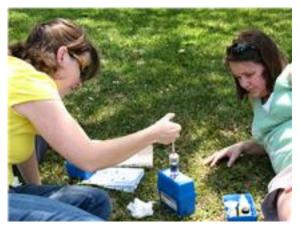
The sampling teams run tests at the five locations on the same date to establish a continuous profile of water quality. The tests are for temperature, pH, conductivity, Dissolved Oxygen and Nitrates. Additional field observations made at the time of each sampling further complete the picture.
