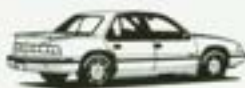
CHEVROLET LUMINA VPV Can use cleaner burning M-85 Methanol resulting in a 30-50% reduction of smog-forming emissions
