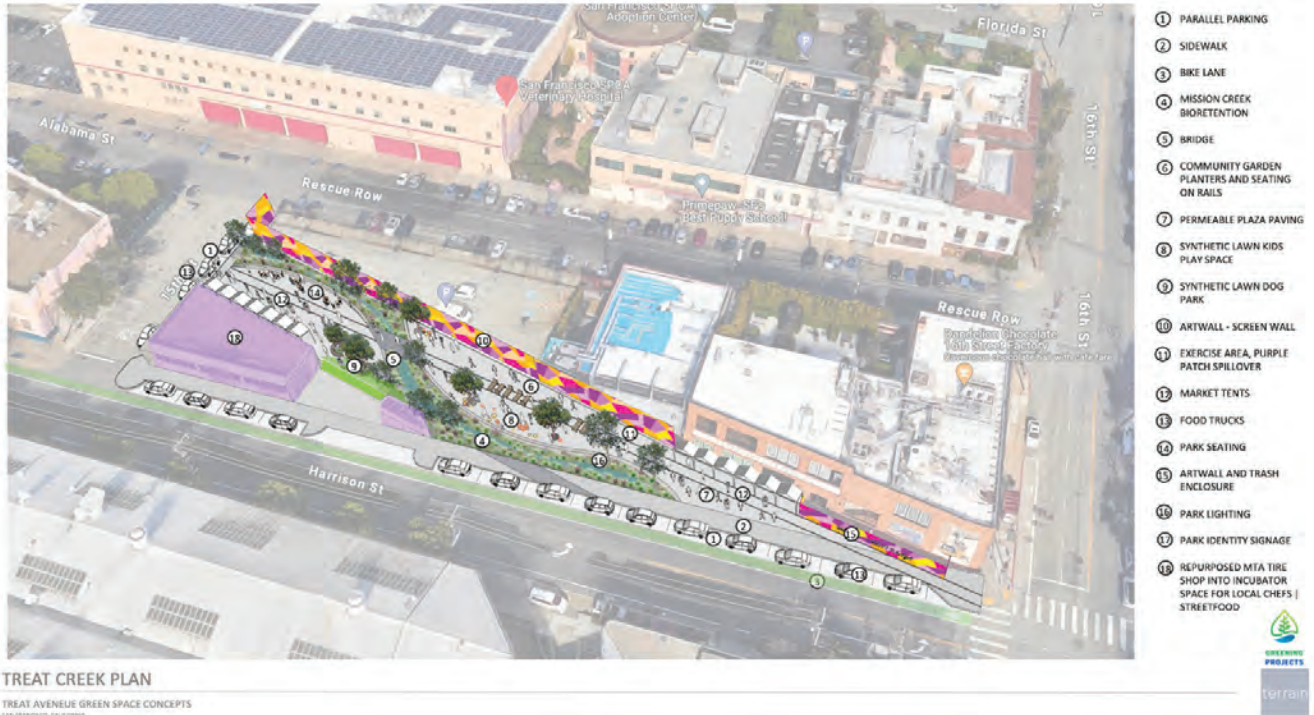
BELOW: Converting an unmaintained street of broken asphalt and polluted wastewater to green, open spaces for the community from Terrain Studio for Treat Plaza North. Illustration for prototype and discussion purposes, not intended as a final engineering design.
