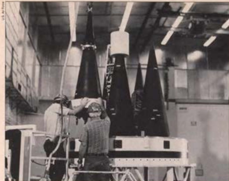
Technicians place nuclear warheads on the nose of an MX. Each missile carries up to 10 independently targeted warheads capable of destroying Soviet missiles in their silos. Opponents fear the MX's power and accuracy could cause the Soviet Union to launch its missiles first.
