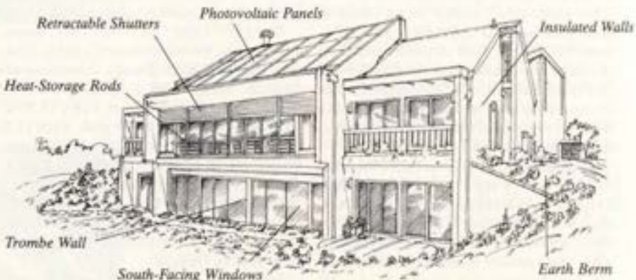
The photovoltaic panels atop Future I make up only part of the home's energy system. Heavy insulation, south-facing double-glazed windows, black-painted heat-storage rods and Trombe wall, insulating earth berms, and retractable shutters reduce the amount of energy needed to keep the house comfortable year-round.
