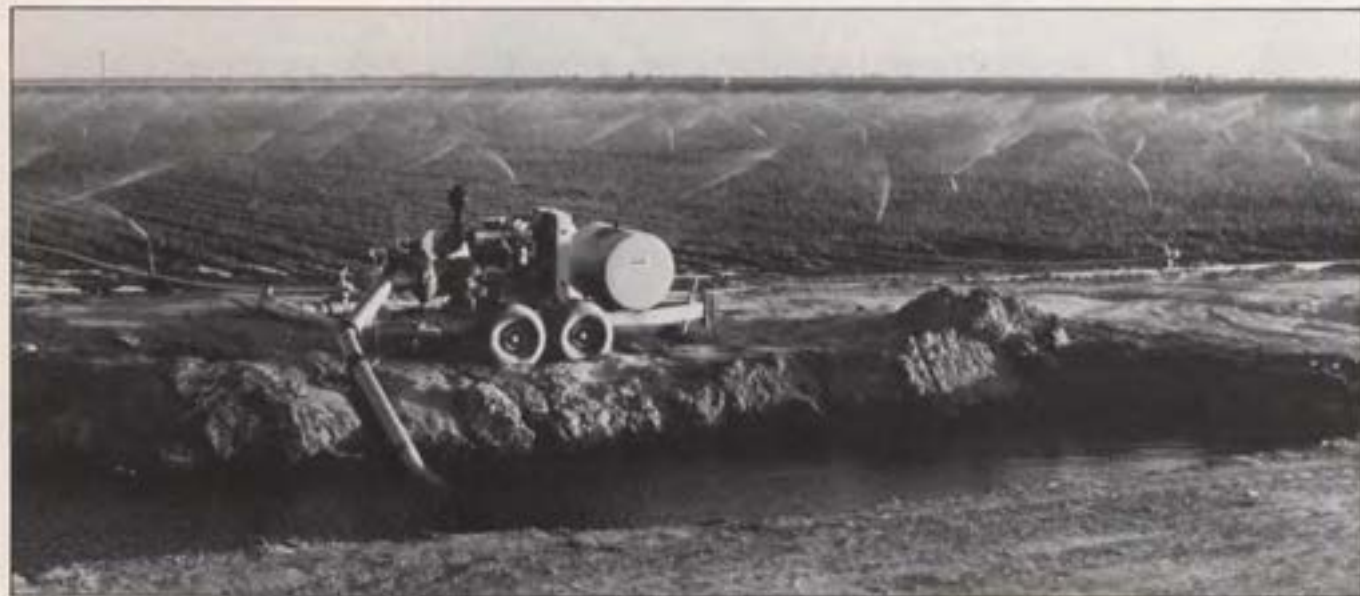
Field hand (left) adjusts the flow of irrigation water to a sugar cane field on the island of Kauai, Hawaii. Portable, diesel-powered irrigation pump (below) drives a sprinkler irrigation system in the San Joaquin Valley in California. The U.S. General Accounting Office estimates that half the irrigation water used in American agriculture evaporates or replenishes the water table without ever reaching the crops for which it is intended.
