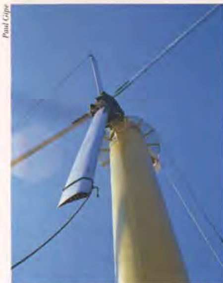
This sophisticated 250-kilowatt wind turbine in Pennsylvania uses airfoils for blades.
