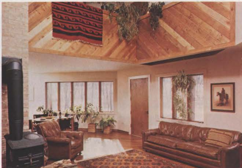
The open floor plan allows air to circulate freely between the floors. The air-lock front entry and triple-glazed windows help to maintain a constant temperature.
