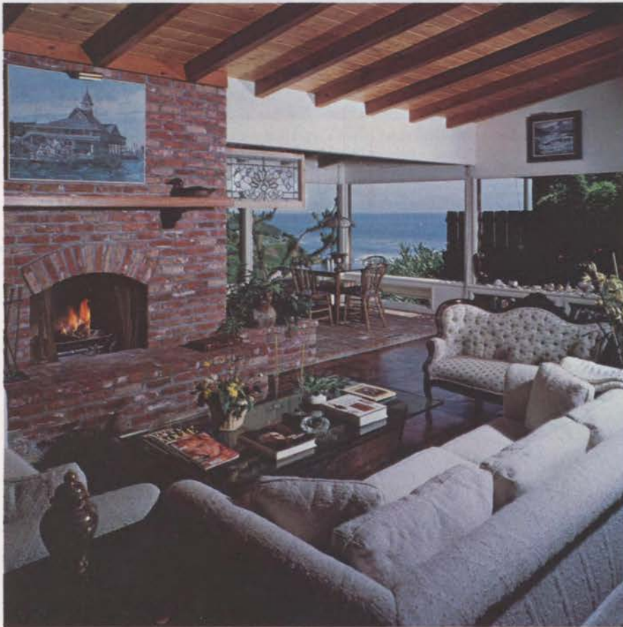
Glass-walled dining area, part of the new brick-floored sun porch, provides a view of the Pacific. Openings below the double-glazed windows admit cooling ocean breezes in summer. In winter, low rays of the sun warm the brick floor and help heat the room.
