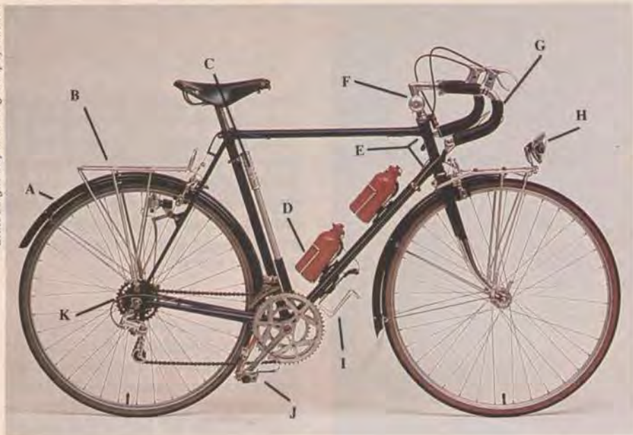
Common bicycle accessories that make touring more comfortable are, clockwise from top left: A—mudguard; B—rack; C—air pump; D—water bottles with cages for attachment; E—lugs (socket-like pieces that join structural tubes; this structural element provides resiliency); F—bell; G—padded handlebars; H—light; I—fuel bottle cage (for camp stove fuel); J—toe clips; K—rear light (on far side of wheel).
