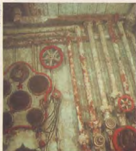
Above left: A diver with underwater camera approaches the impressive propeller of the Henry Chisholm, a 265-foot wooden freighter. Above right: A diver explores the wreck of the America, a small passenger ship that sank in 1928. Above: A gauge panel, steam pipes and valves, festooned with aquatic weeds, aboard the America.
