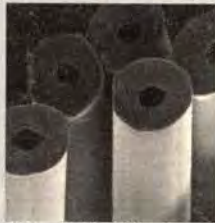
Unique hollow filaments of "Dacron" Hollofil™ II
