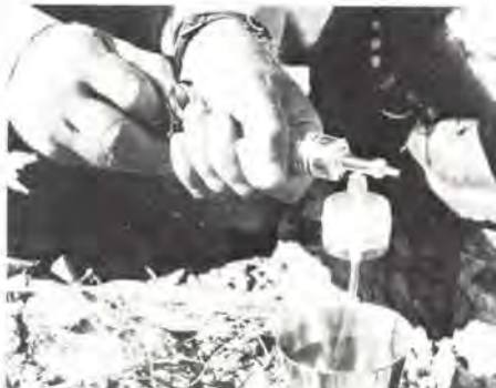
Filtering water sample to check for coliform bacteria
