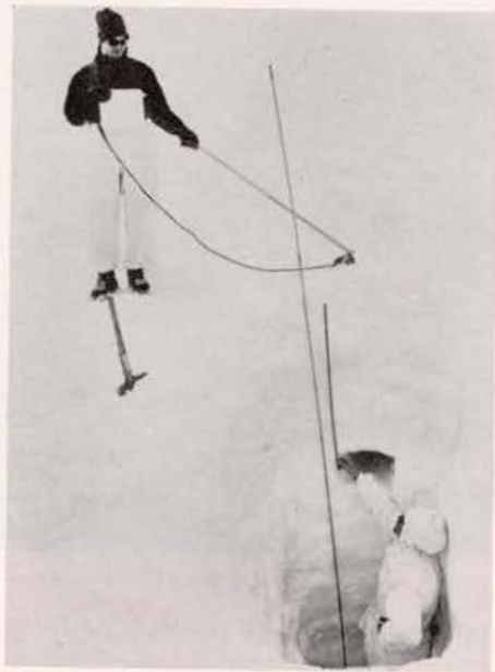
Research scientists took just a few minutes to locate a ski boot buried under several feet of snow, using a Varian portable magnetometer.
