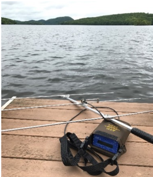
ATS radio telemetry system showing the three element yagi and the R410 scanning receiver. Photo credit: Emily Van Vlack
