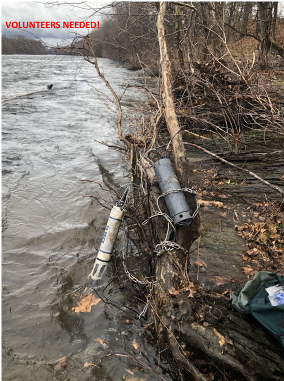
Water quality probe and modem at the Laurys Station monitoring point on the Lehigh
